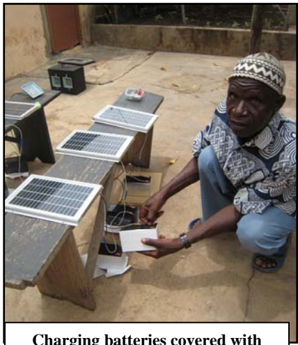
Charging batteries covered with white & silver tape in preparation for performance testing
